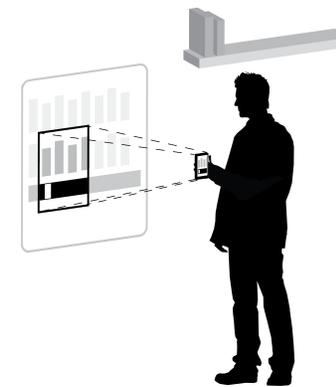
Figure 1: Virtual bookshelf prototype. The user stands in the position of a virtual proximity sensor which launches a virtual bookshelf application on a mobile phone.
